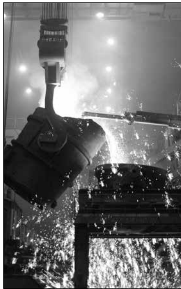
Steel pour during basic oxygen process (photo courtesy of U. S. Steel Corp.).
